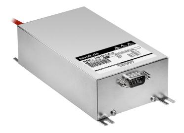
The HMC modules are highly stable, analog controlled high voltage power supplies with fixed output polarity. The HMC series covers output voltages of up to 30kV in a compact metal box. A version in a 3U cassette is available too (HEC series). The maximum output power is 12W.
